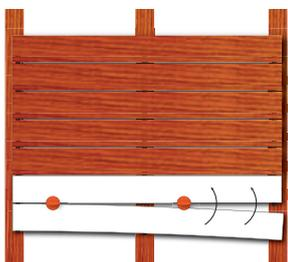
Spacers supplied with the ExtremeKD™ fastener kits are used to prevent crushing the spacer tab when straightening boards.
